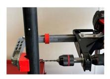
Using Kit #1 with chuck to suit 1mm-13mm twist drills plus holesaws etc.
