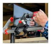
Using Kit #2 with mini cutters from 8mm to 25.5mm Dia.
